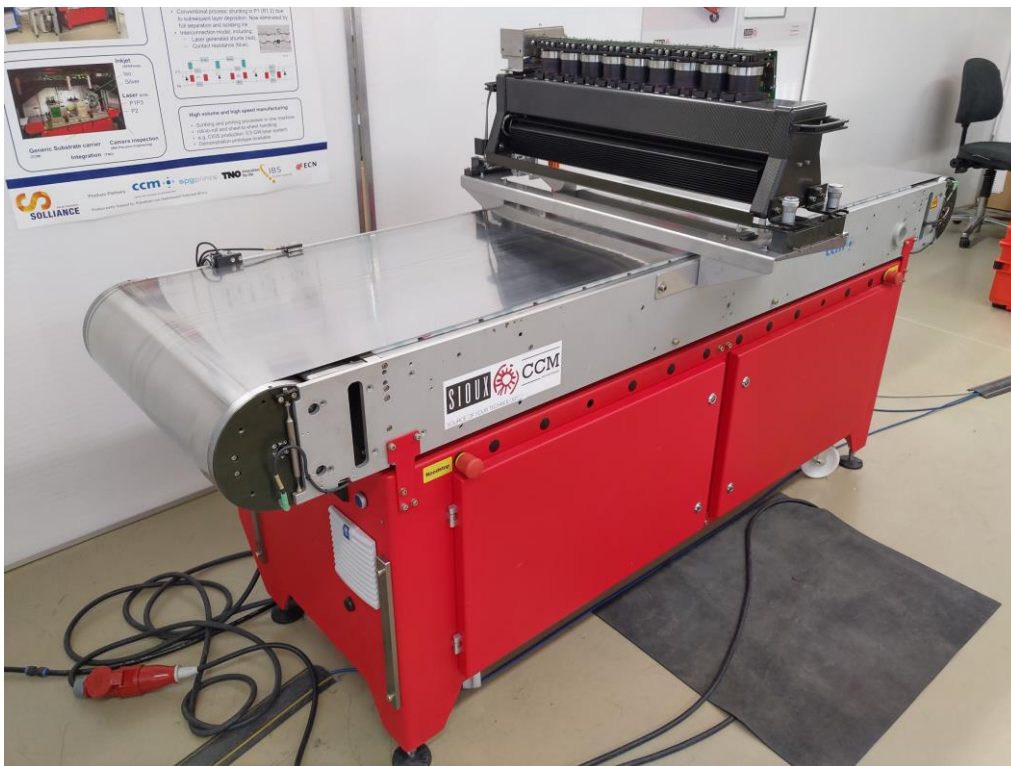
Figure 17: Pilot 1 the generic substrate carrier (GSC)
