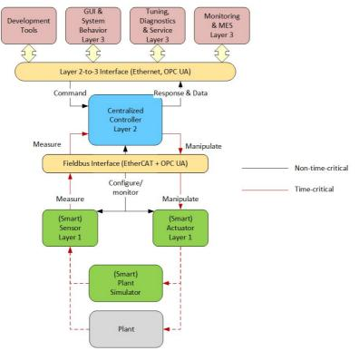
Figure 6 Envisioned layout of the I-MECH reference platform
