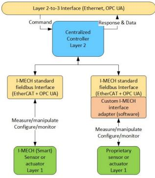
Figure 7 A demonstration of interoperability in connecting proprietary instrumentation layer EtherCAT modules to the I-MECH system, preserving the I-MECH standard interfaces in the control layer.
