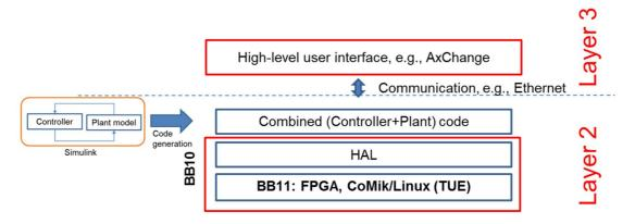
Figure 10 The role of BB10/BB11 in processor-in-the-loop(PIL) testing of the I-MECH reference platform
