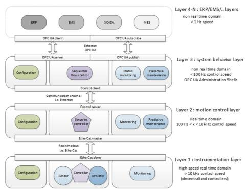
Figure 4 Functional mapping of I-MECH intelligence functions to the I-MECH layers (D6.2).
