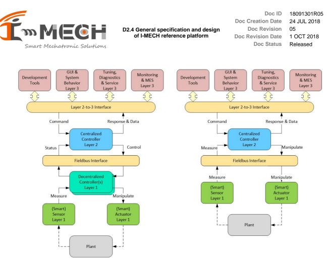
Figure 5 Decentralized (left) and centralized (right) I-MECH platform architectures. The centralized architecture (right) will be reflected in the I-MECH reference platform.
