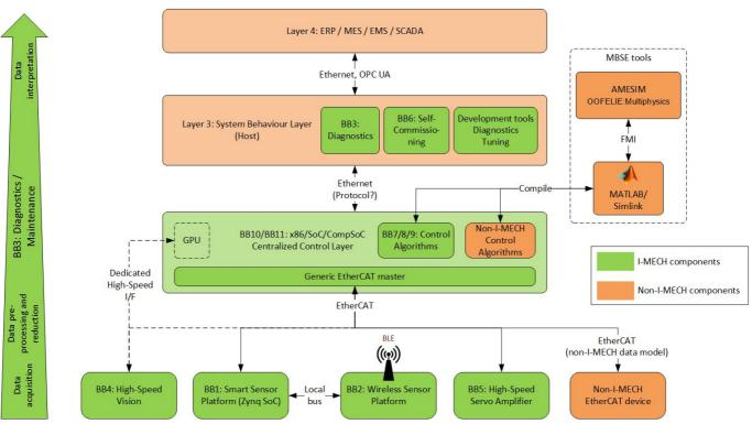
Figure 12 Schematic draft of the I-MECH reference platform architecture. Note that this image only indicates the principal locations of building blocks, whereas actual building blocks have functionalities distributed throughout the system.
