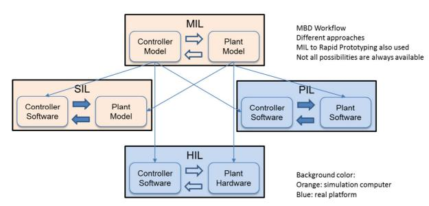
Figure 3 Model-based design workflow as a gradual transition from simulation hardware to real hardware (adapted from WP6 minutes of meeting).
