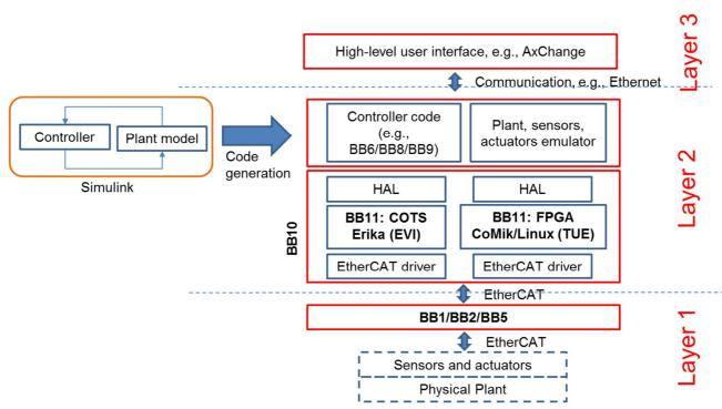
Figure 9 An architectural overview of BB10/BB11 as part of the I-MECH reference platform
