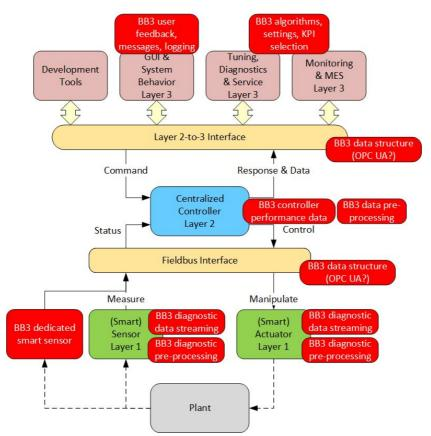
Figure 8 I-MECH reference platform showing the mapping of BB3 (in red) onto the system architecture.
