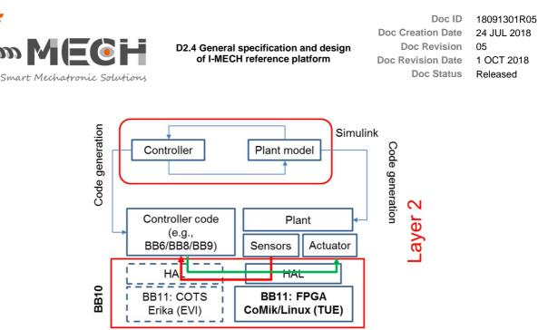
Figure 11 The role of BB10/BB11 in hardware-in-the-loop (HIL) testing of the I-MECH reference platform
